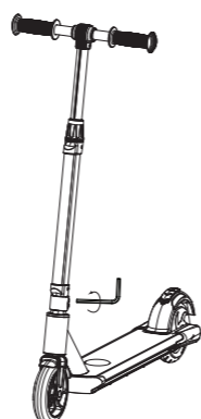
3. Tighten the 2 screws with the screwdriver in package box
